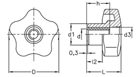
$\begin{array}{ll} D & = 40 \\ d1 & = 17 \\ d3 & = 12 \\ d \ 6H = M8 \\ h & = 18 \\ L & = 27.0 \end{array}$
